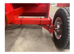
Brake system activated by hydraulic hand pump integrated in the machine with pressure gauge for easy set up to achieve best results when compacting the bag.
