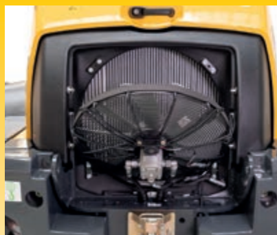
Tiltable radiator fan for convenient cleaning access
